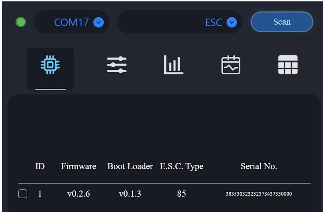
2. Check the power system to be upgraded and click the update upgrade button to select the firmware file.
